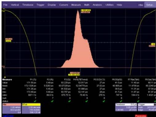
Figure 10 : Trigger link bathtub curve
