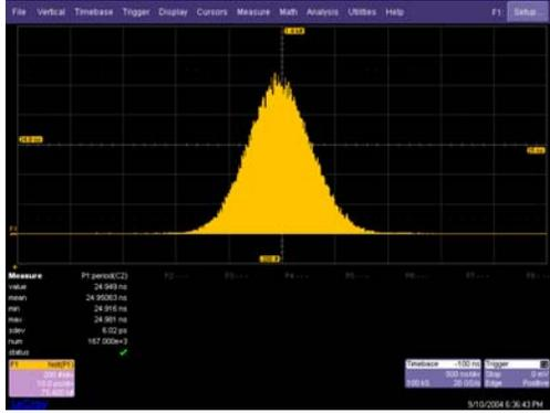
Figure 8 : Jitter measurement
