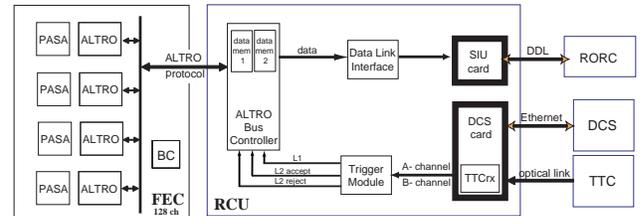
Figure 5: FEE trigger distribution and readout scheme.
