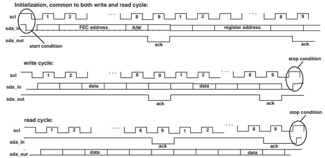
Figure 4: Front-end Control Bus protocol. The standard I<sup>2</sup>C<sup>®</sup> SDA line is split in 2 unidirectional lines: SDA\_in from the RCU to the FECs and SDA\_out in the opposite direction.
