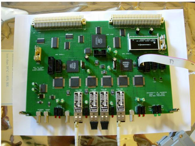
Figure 6: Optical Multiplexer Board.
