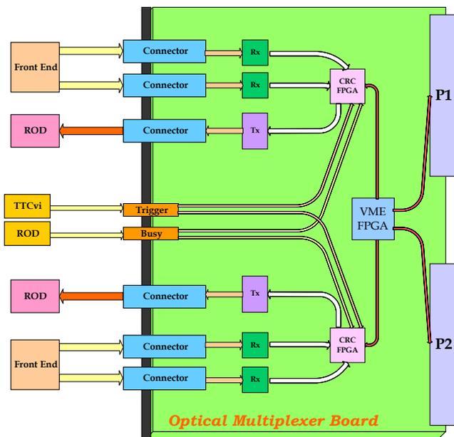
Figure 2: Optical Multiplexer Board Block Diagram.
