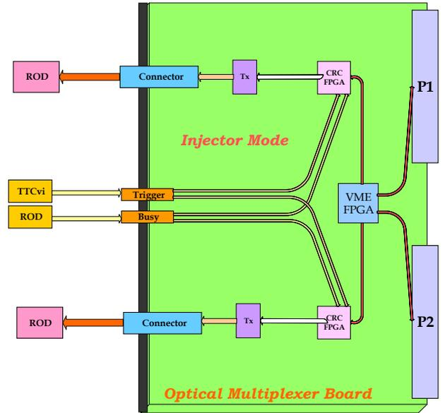
Figure 4: Data Distribution in Injector Mode.
