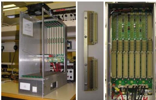
Figure 7: Boundary Scan crate and loop back cards.
