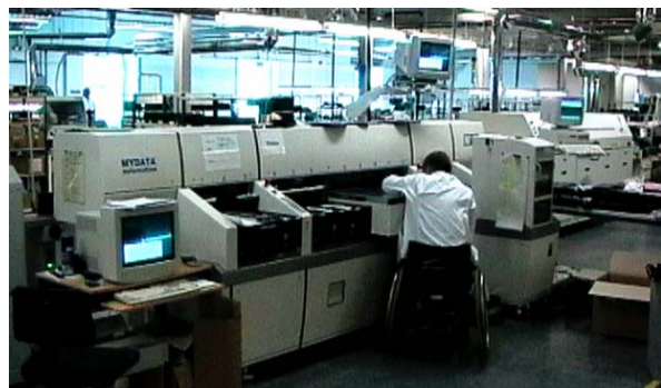
Figure 3: Example of a surface mount assembly line (courtesy DDi Technologies Limited).
