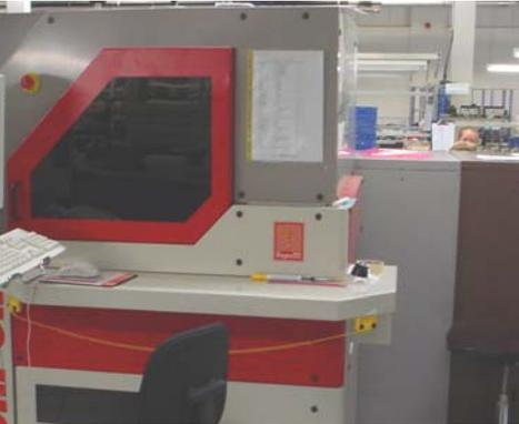
Surface mount assembly checking with Fully Automatic Optical Inspection (AOI) (Diagnosis VisionPoint, ~100 components per minute)
