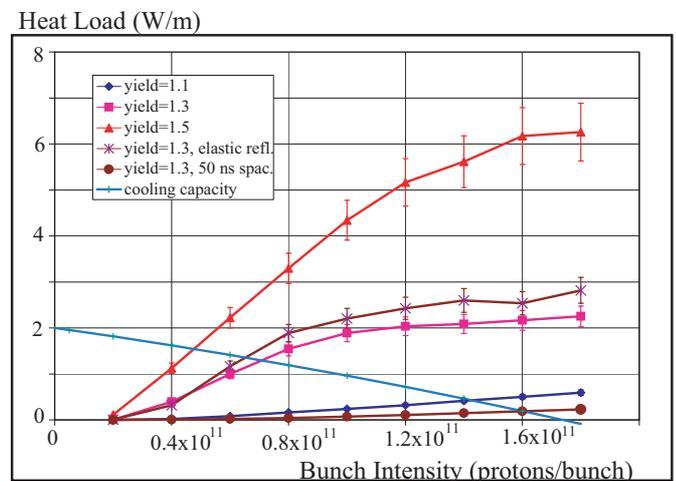
Figure 1: electron cloud induced heat load per meter as a function of the bunch intensity for various bunch spacings and surface properties.
