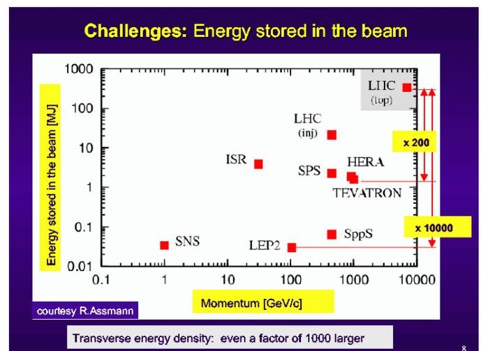
Figure 2: Overview of the stored beam energy and the particle energy in various storage rings.
