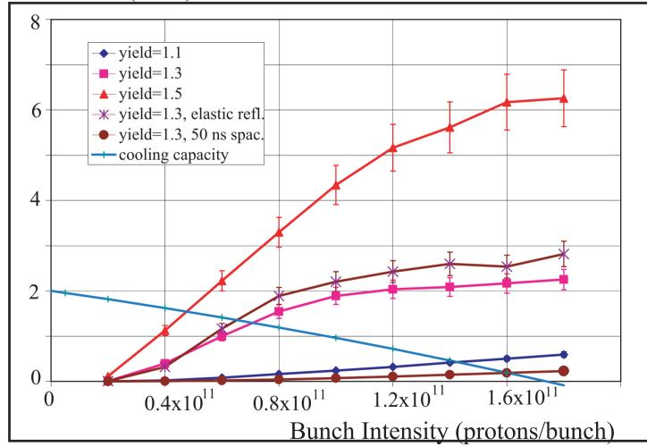
12.5 ns bunch spacing is incompatible with electron cloud induced heat load!
