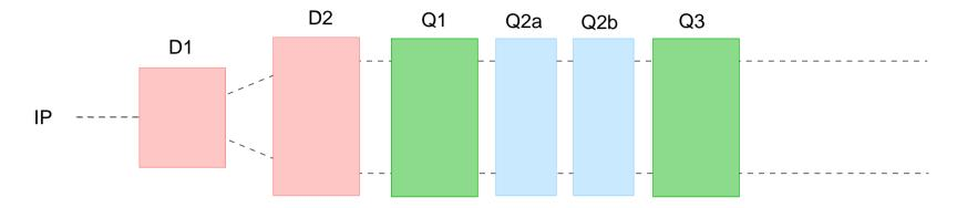
requires radiation hard large aperture D1 dipole magnets
