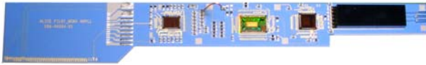
Figure 3: The ALICE SPD MCM. From left to right the Analog Pilot, the Digital Pilot, the GOL and the optical package
