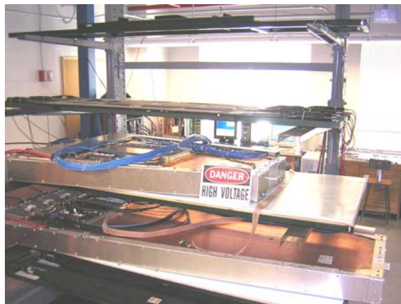
Figure 1: UF Cosmic ray test facility for CSC and electronics
