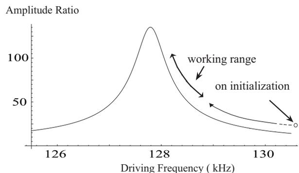
Figure 1: Range of driving frequency for feedback
