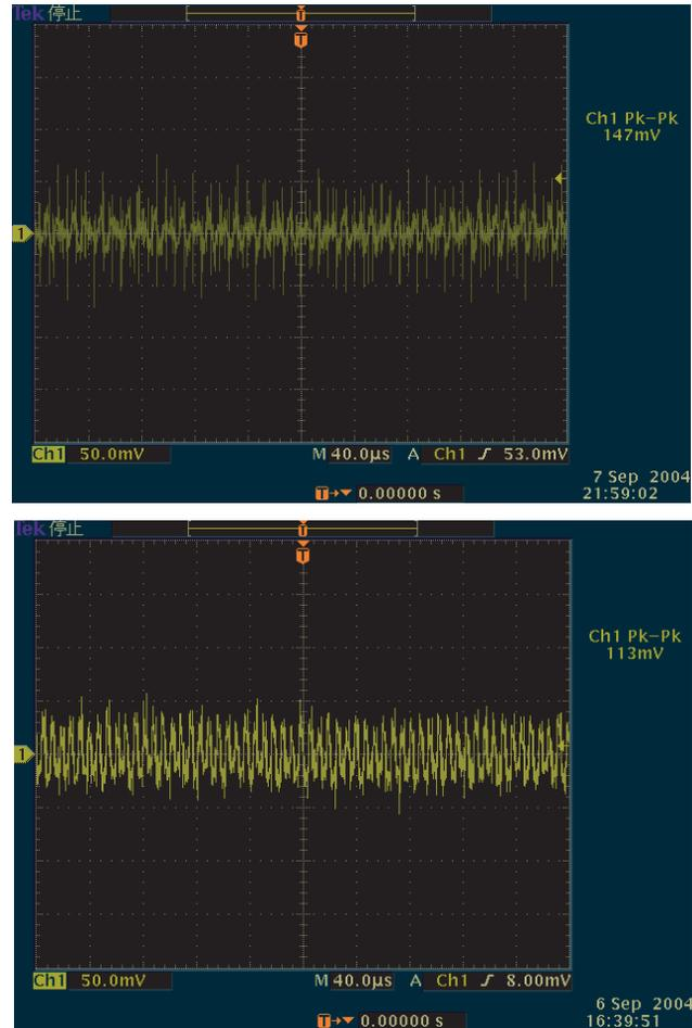
Figure 7: The noise dependence on the load at an output voltage of 3000 V.
