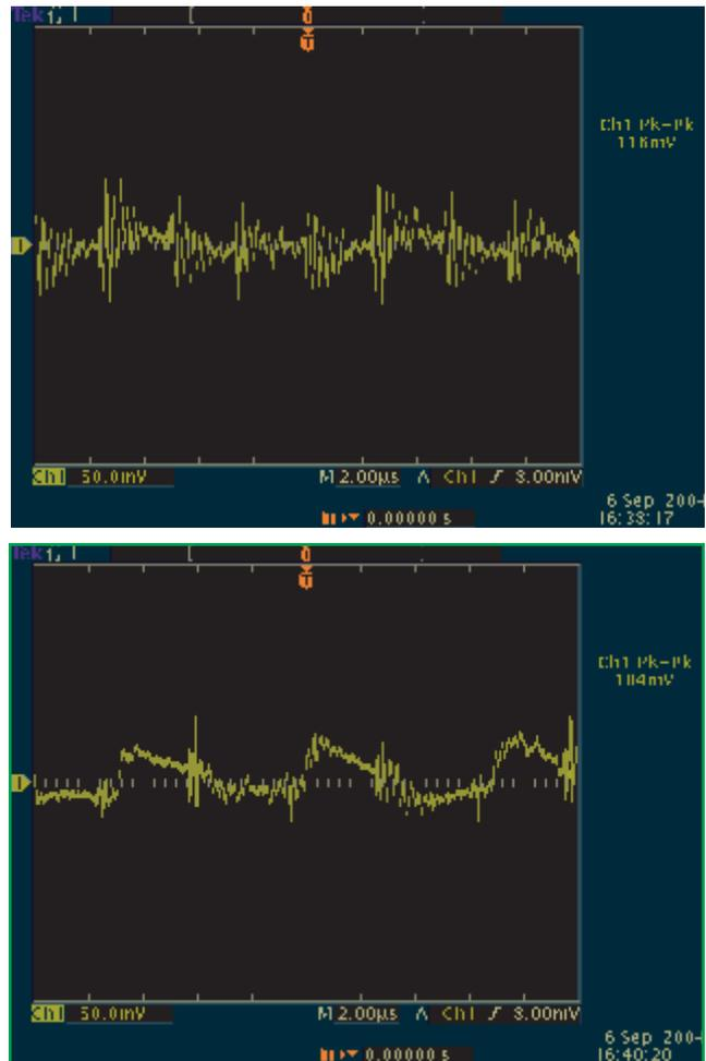
Figure 5: The output voltage from the module is 2000 V at the upper trace and 3000 V at the lower trace where the output voltage is loaded by 25 MΩ.
