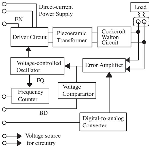
Figure 3: Block diagram of the channel
