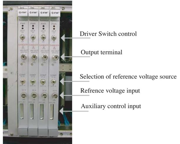
Figure 4: Picture of 4 single channel VME module installed in crate
