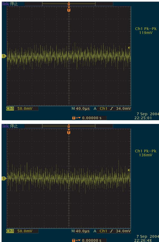
Figure 8: The upper and the lower traces show the output voltages at 2000 V and at 3000 V respectively from the module operating in parallel with other 3 modules where the output voltage is not externally loaded.
