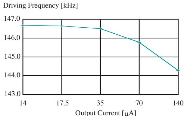
Figure 2: Correspondence between the driving frequency and the output current at an output voltage of 3500 V
