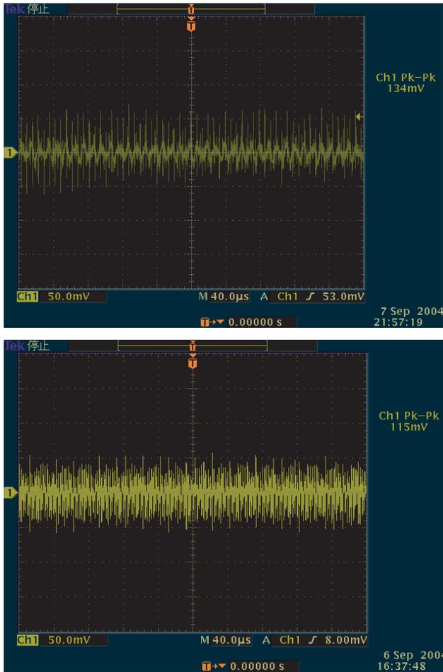
Figure 6: The upper trace shows the output voltage not externally loaded and the lower trace the output voltage loaded with 25 M $\Omega$  at an output voltage of 2000 V.
