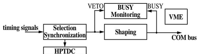
Figure 4: Block diagram of the CTP\_MI module
