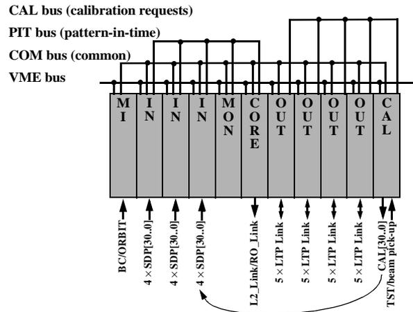
Figure 2: CTP design with its modules, backplanes, and signals
