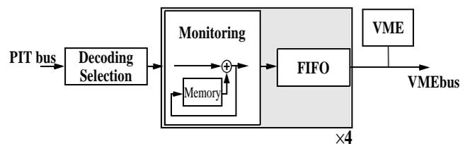
Figure 9: Block diagram of the CTP\_MON module
