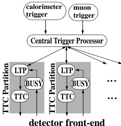
Figure 1: Overview of the ATLAS level-1 trigger
