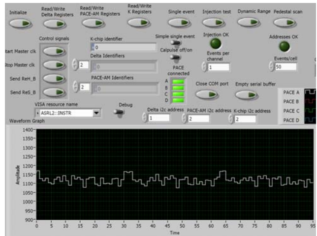
Figure 6: Front panel used to evaluate the CMS Preshower on-detector system board
