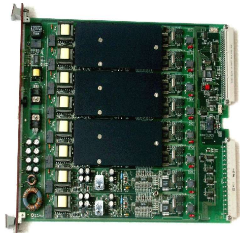
Figure 1. Board with 8 modules of the HV SCT power supplies.
