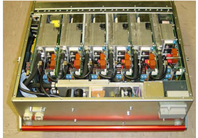
Figure 3: Water cooled PL500 F8, 5 single and 1 dual module
