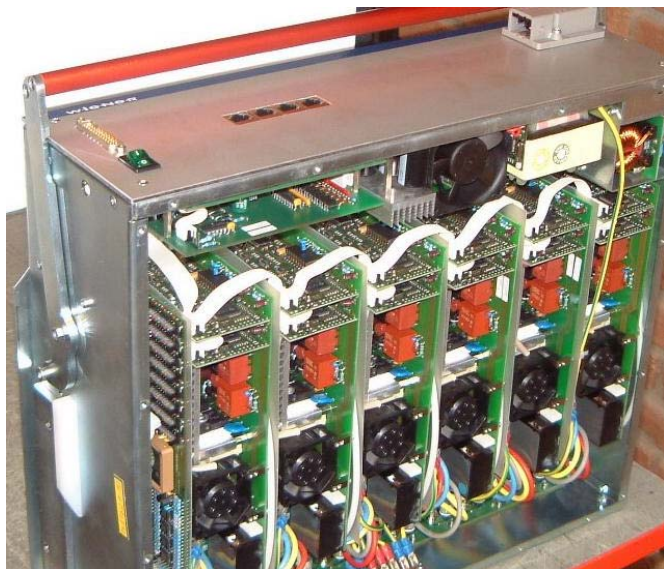
Figure 1: Bottom view of PL500F12, open box with 6 dual modules
