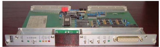
Figure 16. Exemplar of a VME monitoring board for 6 channels
