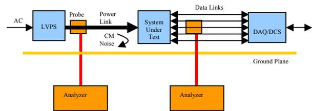
Figure 7: Conducted noise measurement setup.
