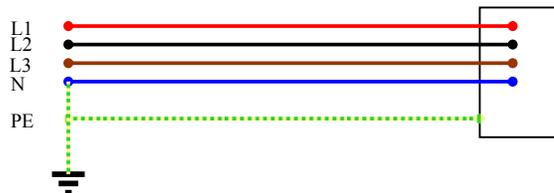
**Figure 1: AC power distribution scheme.**
