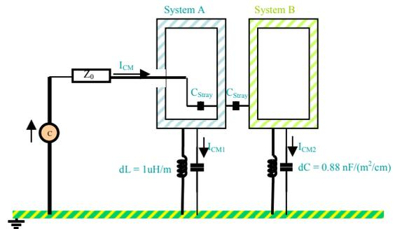
Figure 6: CM circuit model for large systems.
