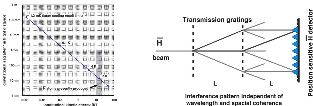
Figure 1: Gravitational sag of  $\bar{\text{H}}$  in the earth field after 1 m flight distance (assuming  $\bar{g} = 9.81 \text{ m/s}^2$ ) and a possible interferometer with two identical transmission gratings and the position sensitive  $\bar{\text{H}}$  detector.
