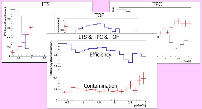
Efficiency of the combined PID is higher (or equal) and the contamination is lower (or equal) than the ones given by any of the detectors stand-alone.
