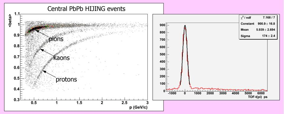
For each momentum p the function r(s|i) is a Gaussian with centroid at  $\theta$  and  $\sigma$  given by the distribution of  $(TOF-t_{\pi})$ ,  $t_{\pi}$ - time calculated by the tracking for the pion mass hypothesis.
