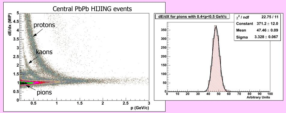
For each momentum *p* the function r(s|i) is a Gaussian with centroid  $\langle dE/dx \rangle$  given by the Bethe-Bloch formula and sigma  $\sigma = 0.08 \langle dE/dx \rangle$
