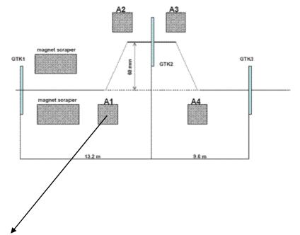
A1÷A4: dipole magnets to provide the momentum selection and recombination
