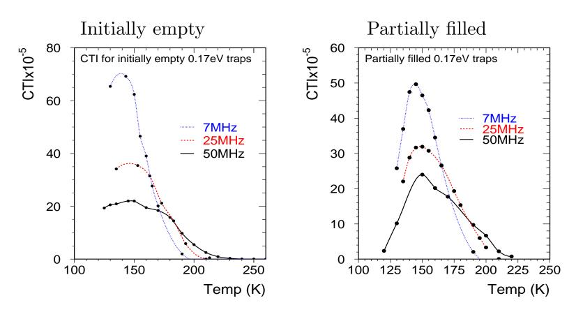
At high temperature: emission time so fast that trapped charge rejoins passing signal.
