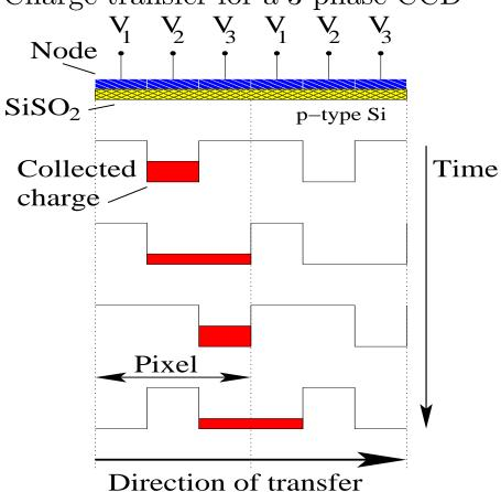
Electrons are collected from ionization of incident particle.
