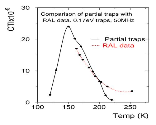
New data will extend temperature range: possibility to measure peak structure.
