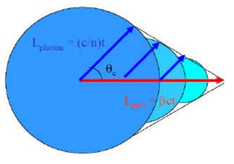
• If a charged particle traverses a medium, at a velocity greater than speed of light in that medium then Cherenkov light is emitted
