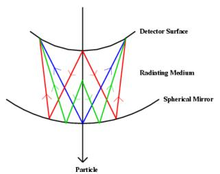
RICH detectors measure angle of emission of the radiation using spherical mirror system
