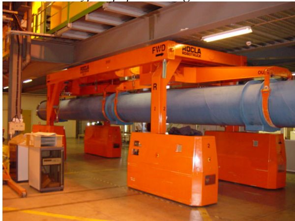
Figure 5: Rocla Cryo-dipole transporters (40 t) in SM18 area
