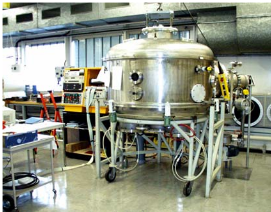
Figures 4a and 4b: New sputter system for the coating of the graphite jaws of the LHC collimators, and view of the sputter source and of the plasma during coating of a mock-up piece
