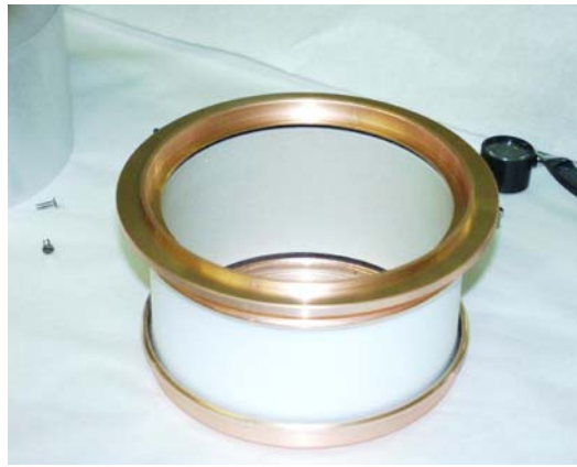
Figure 2: Ceramic windows of LHC main RF coupler after final coating
