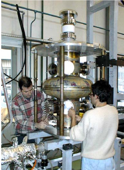
Figures 1a and 1b: First prototype LHC cavity made at CERN and final assembly of a cryomodule containing four superconducting cavities equipped with main RF power couplers
