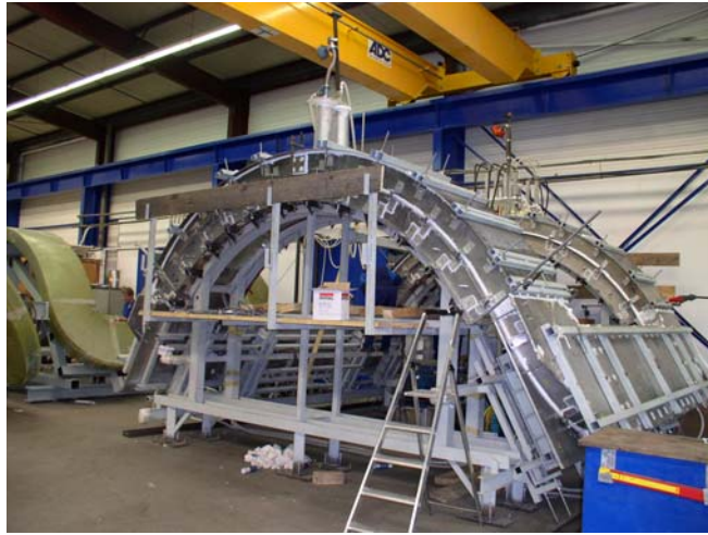
Figure 3: coil impregnation mould for sub-coil 2
