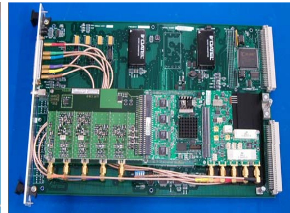
3 rd Generation Field Control Module
