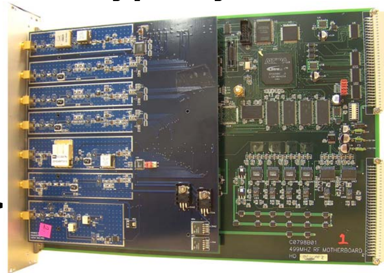
VME Motherboard & 499 MHz Transceiver 2005
