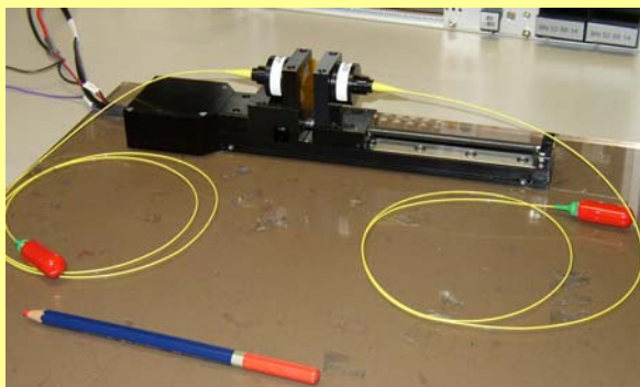
Motorized Optical Delay Line as a phase shifter
