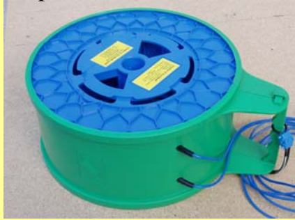
Spool with fiber as a phase shifter
