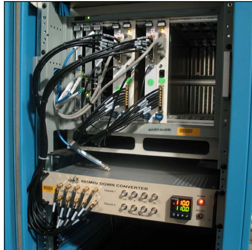
SNS LLRF System using VXI Crate B. Chase, Snowmass05
