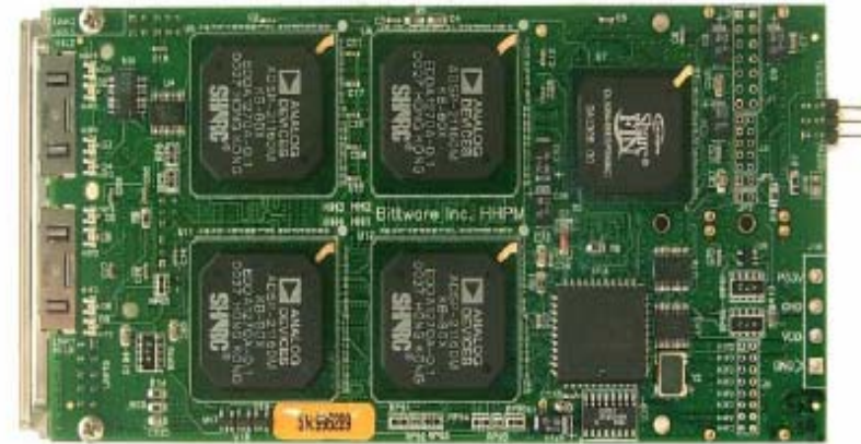
SNS Ring Cavity Controller card S. Peng, PAC05
