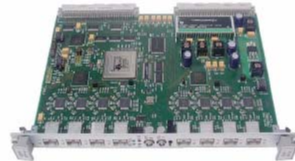
VUV LLRF VME Board V. Ayvazyan et al, PAC05
