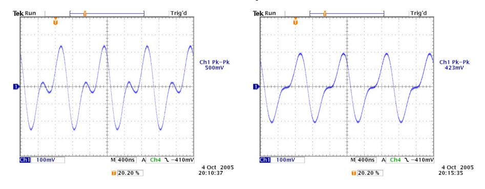
superposition of the harmonics generated by "RFG" module.  $V_4/V_2 = 0.8$  and 0.5. AVC is ON for both harmonics. phase control module is not implemented yet.
