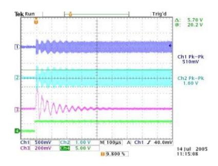
Figure 3: Stable condition:  $X_p = 1$ ,  $X_i = 0.12, X_d = 0$ , external atten- ternal att. 0 dB, the error signal uator -6 dB, the error signal shows shows some ringing no ringing
