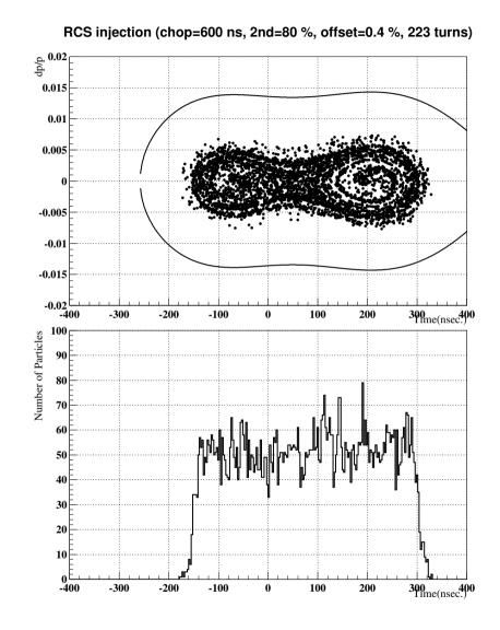
Simulated bunch shape after injection with the second harmonic RF
