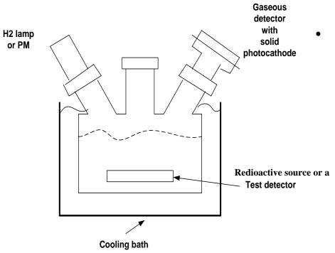
The second set up was a chamber which could be immersed into the bath cooled with the LN<sub>2</sub> or other liquids. It allowed several independent studies to be carried out, for example, detection of the scintillation lights from (175 nm) LXe by a PM or by a gaseous detector with CsI photocathodes.
