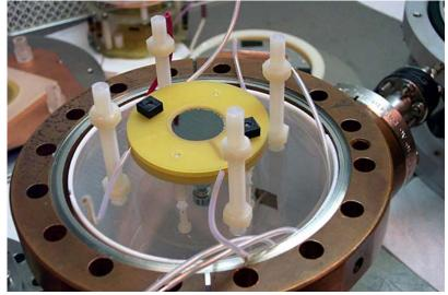
A chamber which could be immersed to the bath cooled with LN<sub>2</sub> or other liquids
