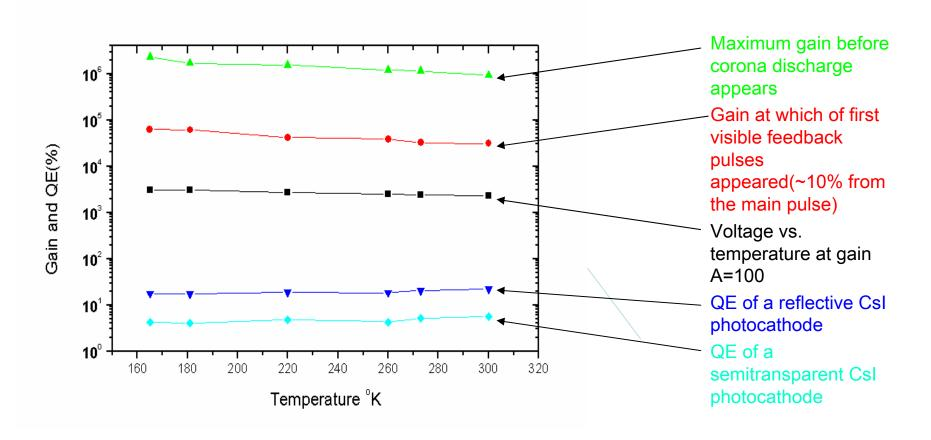
The QE of these photocathodes both in the vacuum and in a gas at some temperature intervals, including those which corresponded to LXe or LAr. For this a pulsed H<sub>2</sub> or a continues Hg lamp, was used with a system of UV filters. The absolute intensity of the light beam was measured by a calibrated Hamamatsu vacuum photodiode and the calibrated CFM-3 counter. See for detailes **physics/0403087** February 2004.
