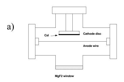
In case of semitransparent CsI photocathode It was was evaporated on the MgF<sub>2</sub> window.
