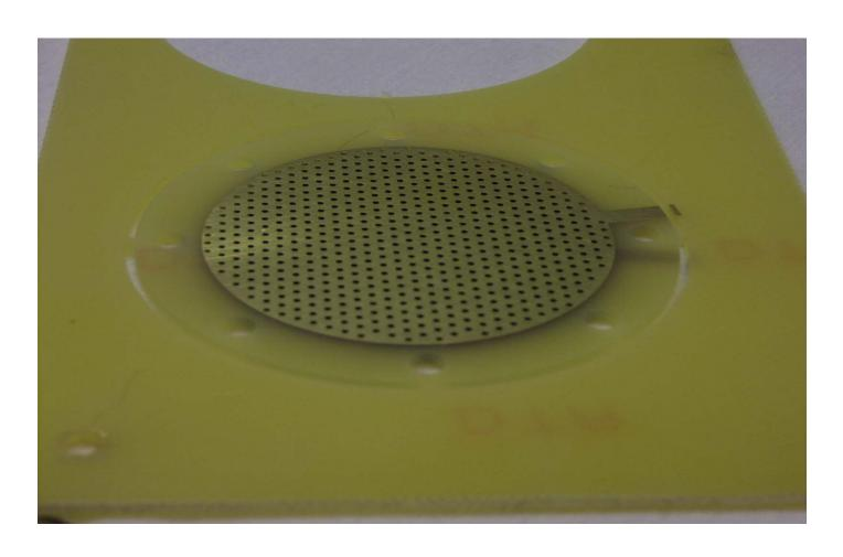
Circut board G10, with drilled holes, coated with Csl.
