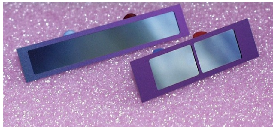
first 'dummy' samples: 50µm silicon with 350µm frame
