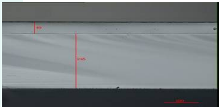
Electron micrograph of cut through bonded and thinned wafer
