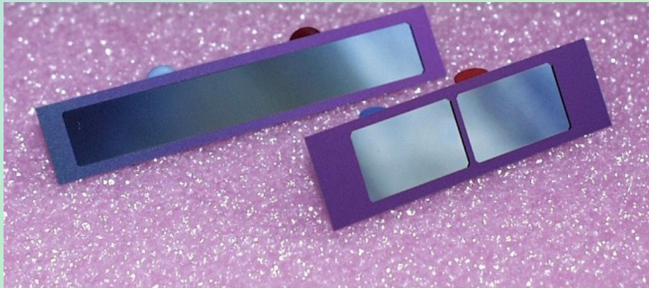
first 'dummy' samples: 50µm silicon with 350µm frame
