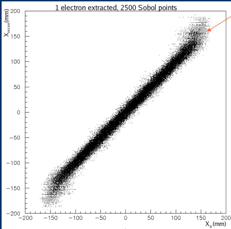
Even with only 1 e- extracted from the liquid ( $\sim$ keV NR), we are able to reconstruct up to the edge of the PMT array ( $\sim$ 160 mm)
