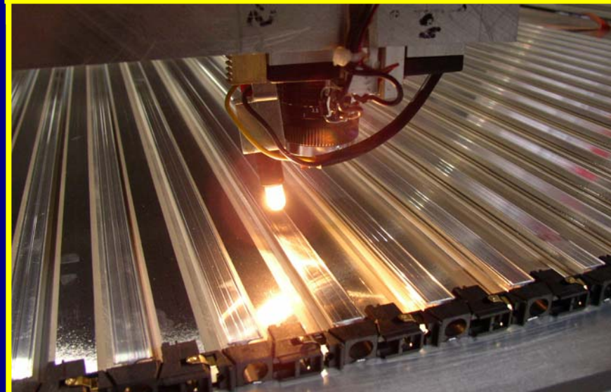
Wire positioning and measurement (precision of 100 \mu\text{m} required by trigger)
