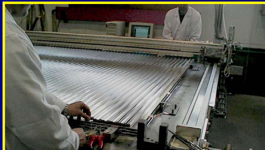
Wire positioning and measurement (precision of 100 \mu\text{m} required by trigger)
