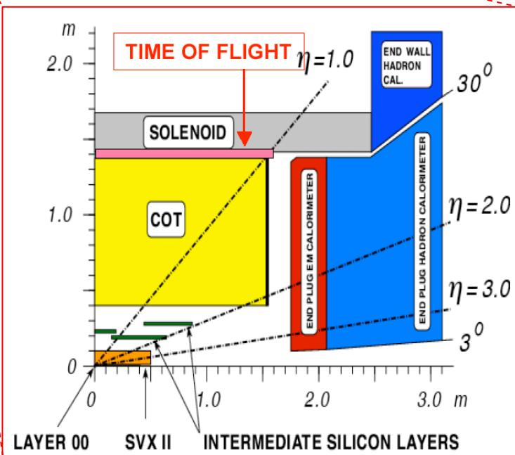
**LAYER00** 1 radiation-hard silicon layer at  $R = 1.5$  cm.
