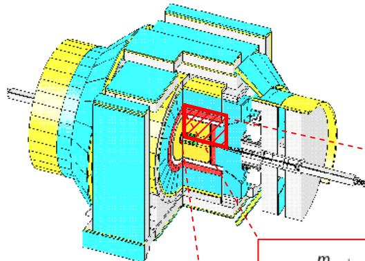
**Muon** 4 layers of single wire drift cells
