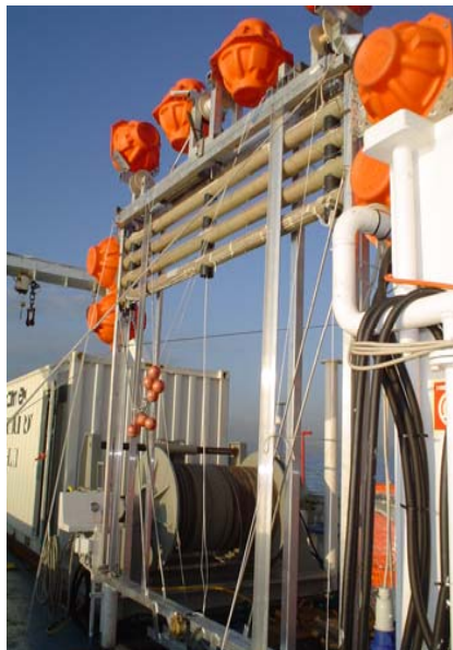
A 1:5 scale model of the tower – 4 floors tested in shallow water (April 2004)
