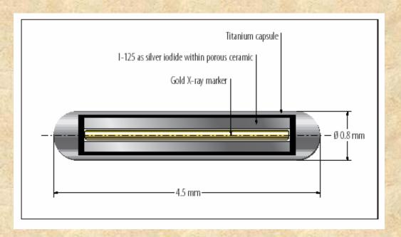
The IsoSeed is equipped with a high-density gold marker providing excellent CT visibility. The full-length marker allows easy and precise location of each seed and produces minimal artefacts. This enhances the precision of the post-implant quality control.
