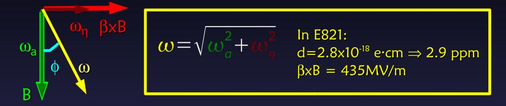
Tilt in precession plane:  $\phi \cong \omega_{\eta}/\omega_{a} = \eta \beta/2a$  $S_{v} \cong S_{0} \phi \sin(\omega_{a}t) \qquad S_{L} \cong S_{0} \cos(\omega_{a}t)$
