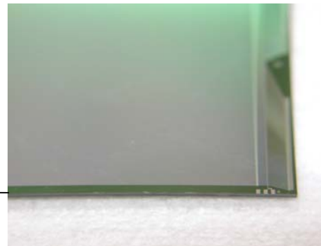
Detail of 3x4 cm 2 Totem Planar/3D Detector fabricated within P324
