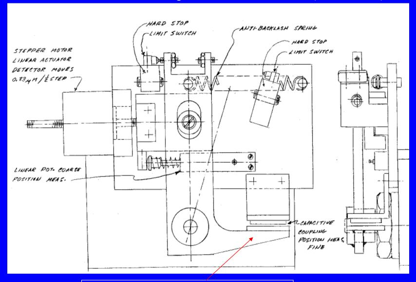
Gap measured capacitatively → position
