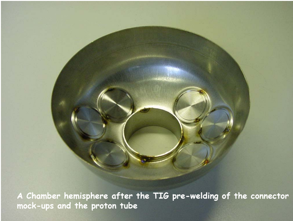
Concave forms are difficult for TIG welding. A welding lip is clearly seen on the left against the tube
