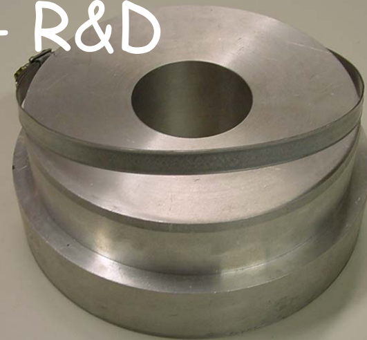
The welding jig used in the chamber cylinder welding
