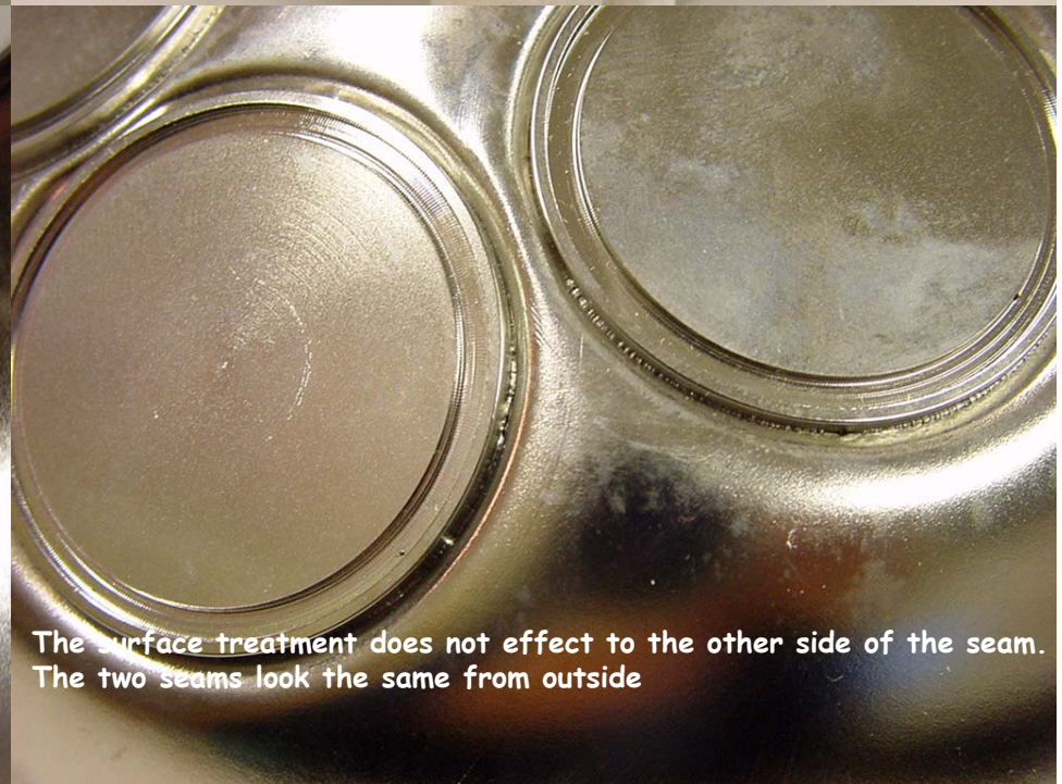
Normal fitting produced a perfect seam
