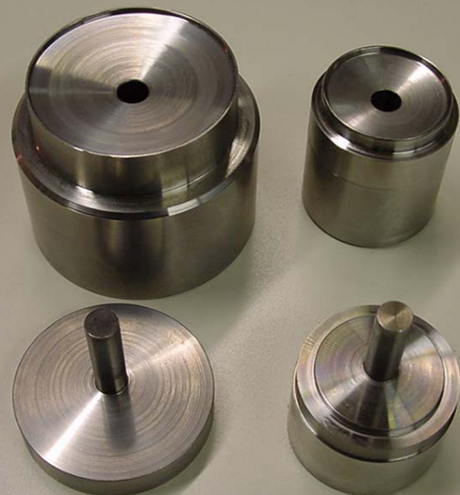
Pressing tools for the proton tube and connector welding lips
