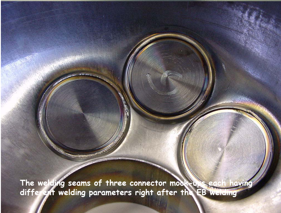
A Chamber hemisphere after the TIG pre-welding of the connector mock-ups and the proton tube
