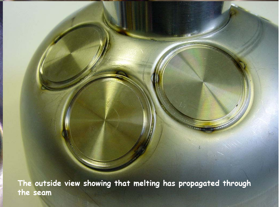
Concave forms are difficult for TIG welding. A welding lip is clearly seen on the left against the tube
