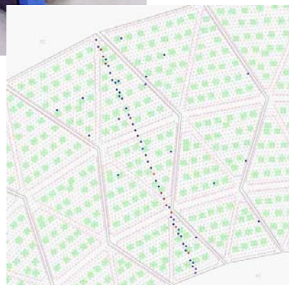
Cosmics muon in assembled barrel TRT
