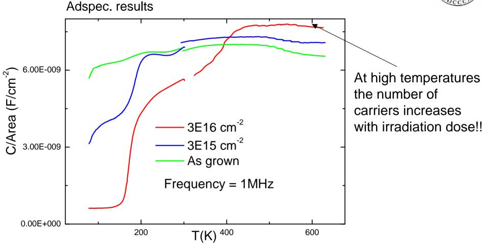
The steps tell us that the compensation at lower temperatures is caused by deep levels. No deactivation observed.
