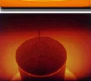
5. Conical tail growth after completion of body.
