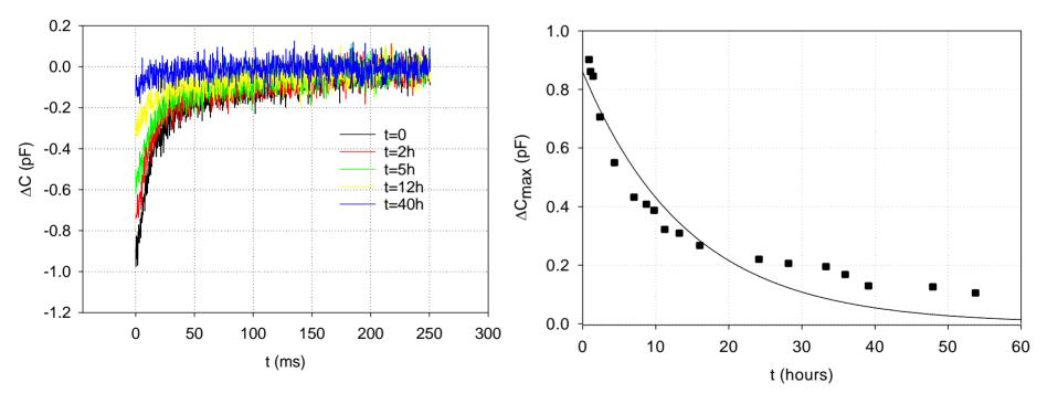
Note: The samples were copper contaminated over a year ago, copper is still in the interstitial form. Corona charge is very effective in preventing out-diffusion!
