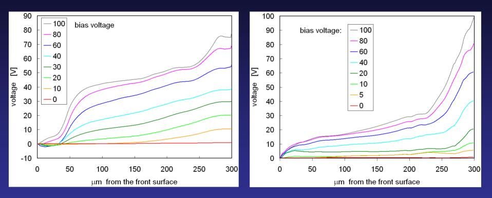
1 MeV neutron equivalent fluence of 1.09E14 /cm2 . 1 MeV neutron equivalent fluence of 6.45E14 /cm2 .
