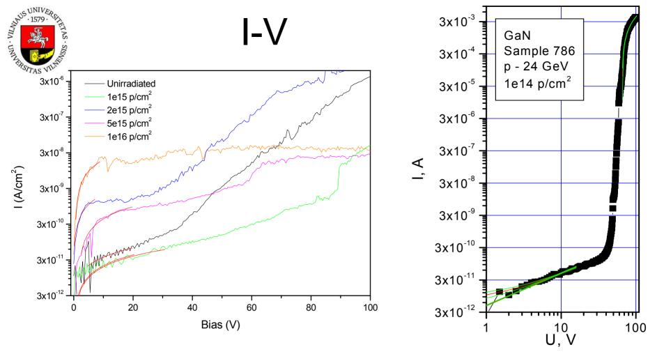
At low bias dark current liner depend on bias – *the red lines linear dependence fit.*
