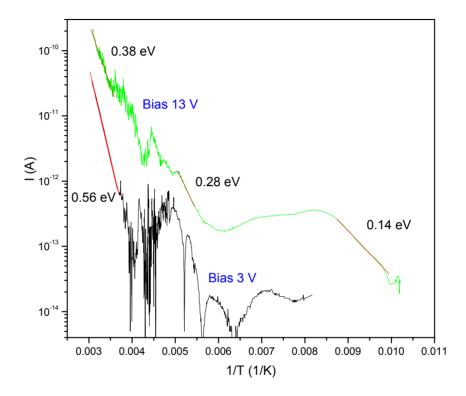
The characteristics measured at different bias additionally demonstrate the existance of instabilities related to the percolation through the inhomegenities in the sample. These inhomogeneities are similar as was observed in the thin samples and are related with the structural defects (influenced by irradiation).
