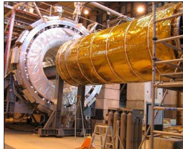
Solenoid just before insertion into the cryostat
