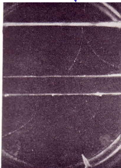
Production of an electron-positron pair by a high-energy photon in a Pb plate
