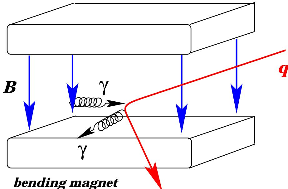
→ ■ ***radiation fan in bending plane***
