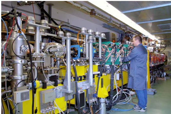
Bunch length adjustment with magnetic chicane
