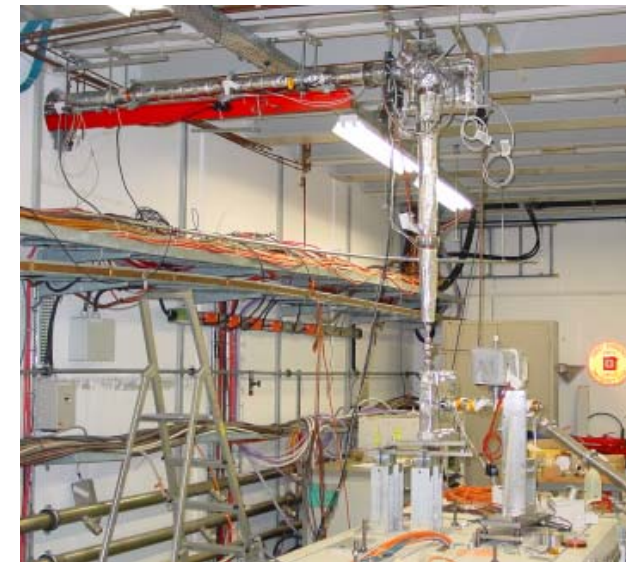
17m waveguide with 5 bends but low-loss (85% transmission) (Russian collaboration)
